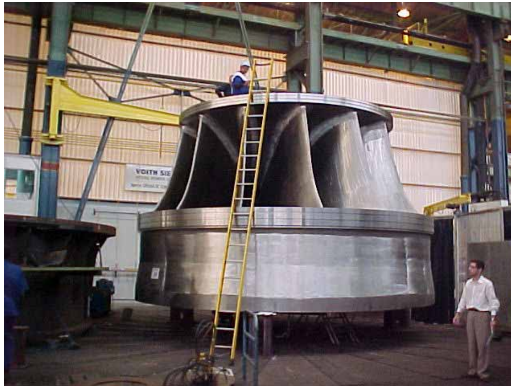
Prototype runner at the manufacturing shop.
