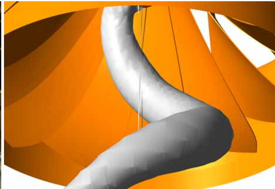
Numerically simulated for part load at low head (vapour pressure isosurface)
