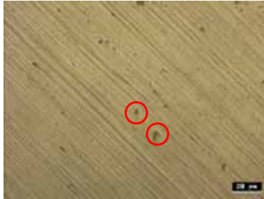
Microscopic picture of 316L after electrochemical treatment
