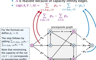
Note that minimizing the capacity of the cut  $(A, V \setminus A)$  corresponds to maximizing profits of projects in A.
